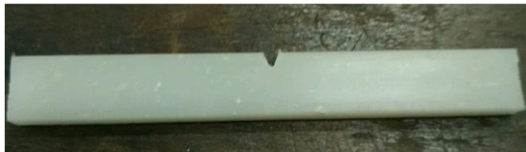
Figure 2. Impact test specimen.
