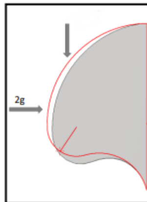
Figure 15. Gravitational influence and additional force to simulate a shrinkage movement. The red line represents the pre-gravitational influence geometry and the grey solid line represents the post-gravity influence geometry.
