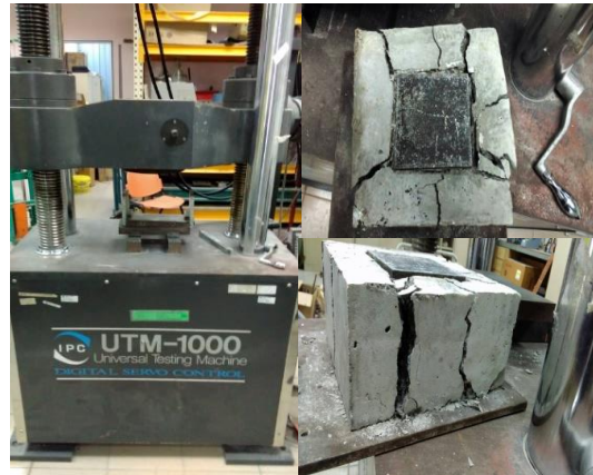
Figure 2. Bearing Strength Test
