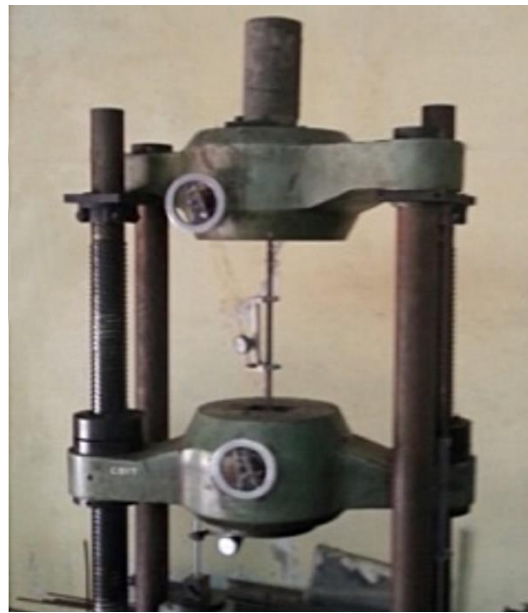
Figure 2. The test set up for pull out test
