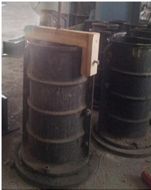
Figure 1. Cylindrical moulds with a wooden channel to support steel rod
