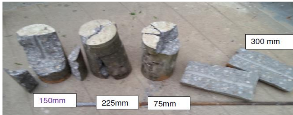
Figure 6. Splitting Modes of failure for 16 mm diameter bars embedded into various lengths of M60 concrete cylinders with 50% RCA.
