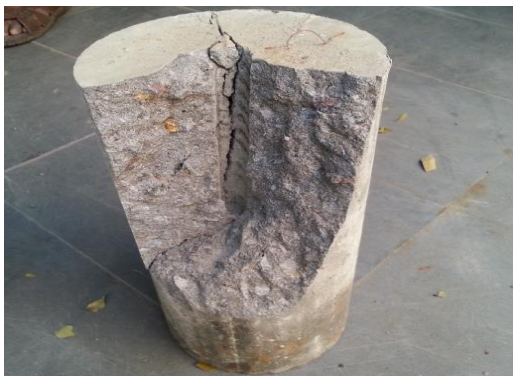
Figure 3. Splitting failure for 16 mm dia. bars embedded up to 150 mm in M60 concrete
