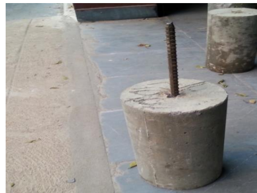
Figure 4. Steel rupture Mode of failure for 12 mm diameter bars embedded to 300 mm.
