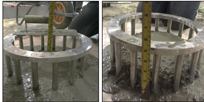
Figure 1 : J-ring test (a) Plain SCC (b) SCCFibre
