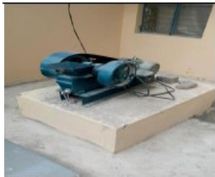
Figure 4. Demolished Concrete Material and Laboratory JAW crusher
