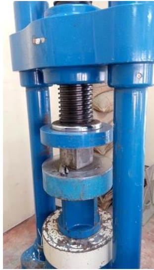
Figure 5. Testing of cubes in UTM
