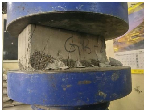
Figure 3. Compressive Strength Testing on Geopolymer Brick.
