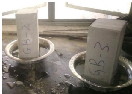
Figure 7. Efflorescence of Bricks.
