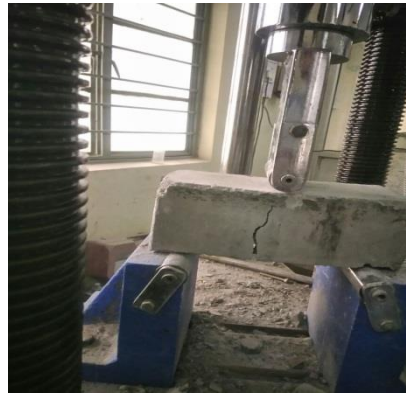
Figure 5. Flexure Strength Testing of Brick.
