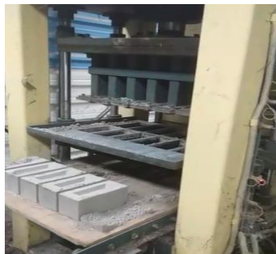
Figure 1. Manufacturing of geopolymer bricks.
