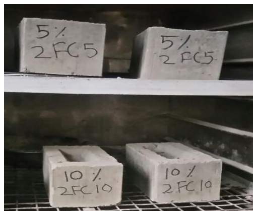
Figure 2. Typical Geopolymer Fly Ash Brick.
