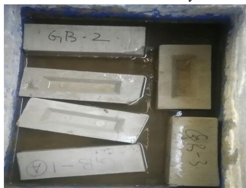
Figure 6. Water Absorption of Geopolymer Bricks.
