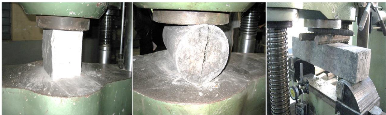
Fig. 3: Compressive strength test Fig. 4: Split tensile strength test Fig. 5: Flexural strength test
