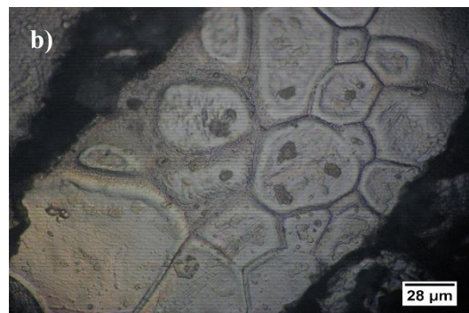
Figure 8: Optical microscope images ageing sample at 6 hours a) AZ91 b) AZ91+0.3% CNT.
