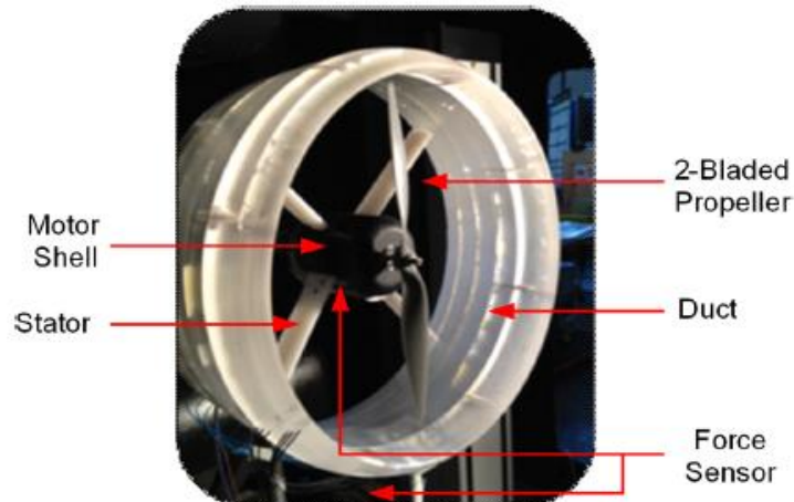
Figure 1. Ducted propeller (mouth-ring) [5]
