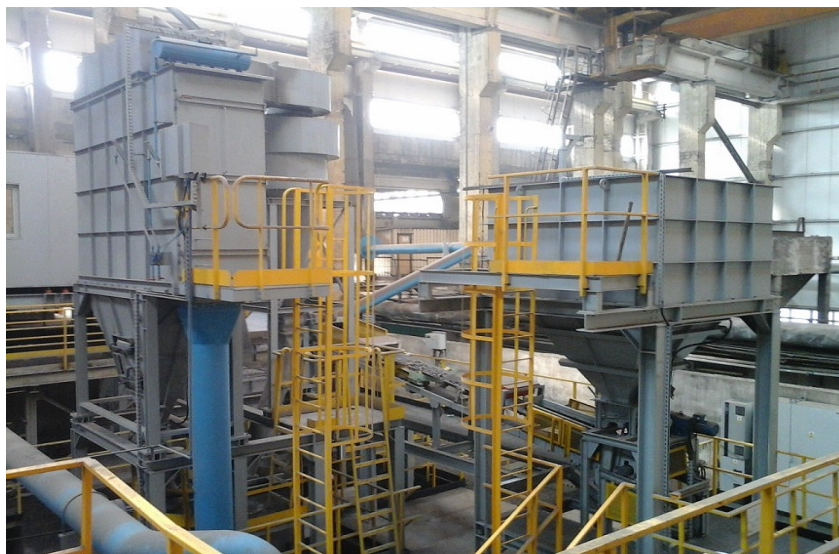
Figure 4. View of the pilot installation preparing ore for flotation using the impact comminution technique in Lubin Ore Enrichment Plant.
