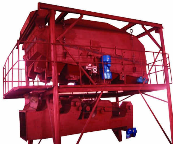
Figure 3. Air jig TFX unit [14].
