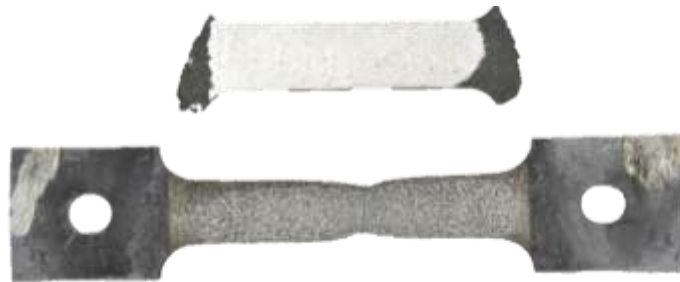
Figure 10. Sample B after the shear-tensile test.
