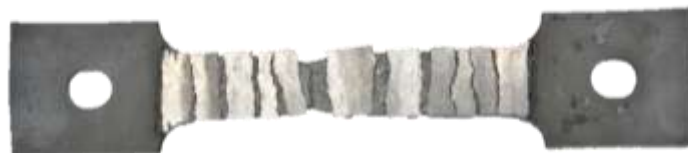
Figure 11. Sample C after the shear-tensile test.
