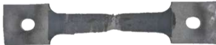
Figure 14. Sample F after the shear-tensile test.
