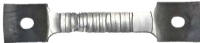
Figure 13. Sample E after the shear-tensile test.
