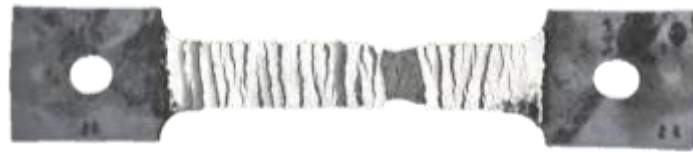
Figure 9. Sample A after the shear-tensile test.
