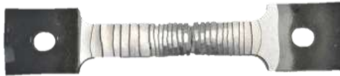
Figure 12. Sample D after the shear-tensile test.
