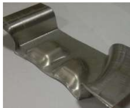
Figure 2. Industrial part: wing stiffener applied for comparison of experimental and numerical modelling results
