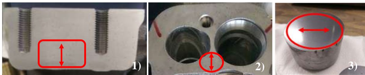
Figure 2. The investigated areas of the experimental castings (1, 2) and the thermal analysis sample (3)
