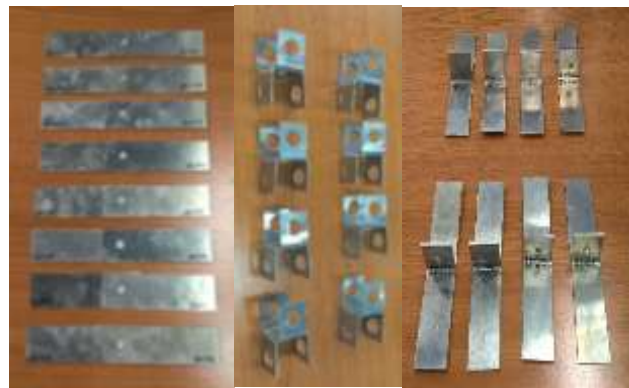
Figure 9. The samples used for tensile, head pulling and neck pulling tests.
