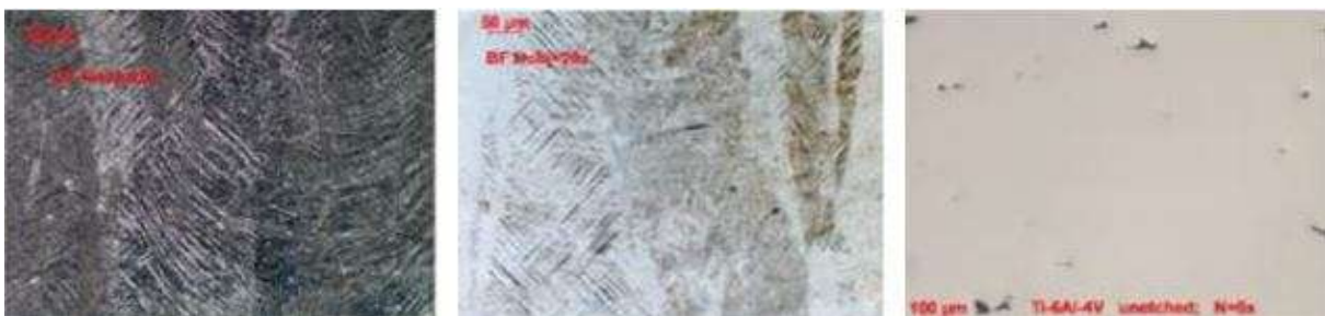
Figure 5. Grain structure of 3D-printed titanium samples
