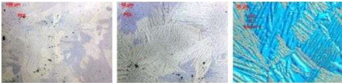
Figure 4. Grain structure of cast titanium samples
