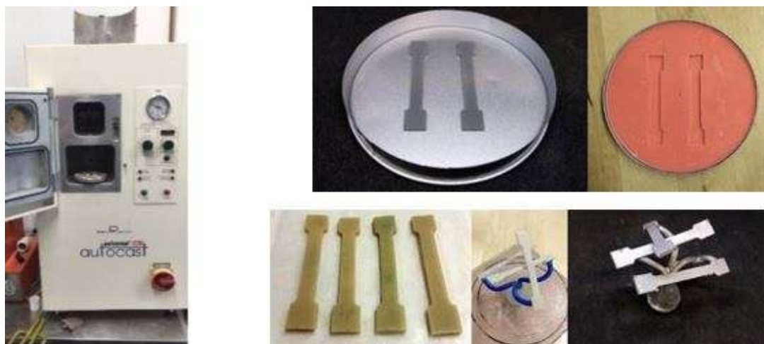
Figure 1. Manufacturing steps of titanium alloy specimens at casting processes
