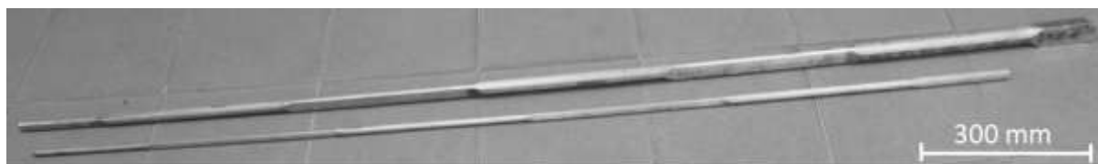
Figure 1. The examined strand in two pieces including all the technological steps
