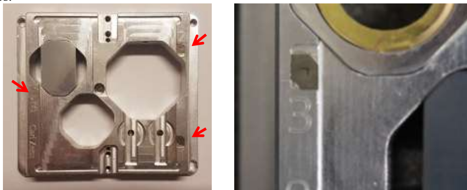
Figure 1. Zeiss sample holder with markers for correlative microscopy
