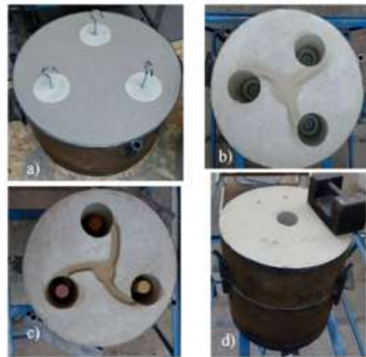
Figure 2. The experimental moulding box, a) lower part with the cores, b) tangential access channel without cores and c) with core d) lower and upper moulding box with weight on
