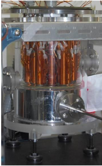
Fig. 6: Experimental apparatus for stirring of molten gallium.
