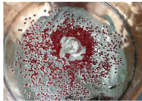
Fig. 13: Particle “slag” distribution; h_0=20\text{mm} , I_{\text{rms}}=1000\text{A}
