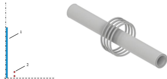
Figure 2 – Case 2.0: 3D rendering of the tube and the coil (right) and the scheme of 2D axially symmetric system (left). On the scheme: 1 – the tube, 2 – the coil.
