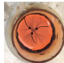
Fig. 8: Photograph of inductively stirred vanadium oxide melt.
