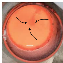
Fig. 7: Photograph of inductively stirred NaCl-KCl melt.
