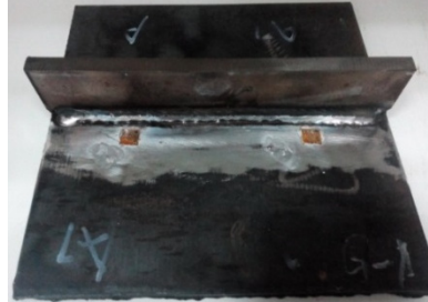
Figure 1. The residual stress measurement of T-joint
