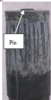
Figure 3. Brittle fracture of the pin
