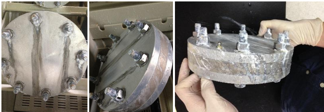
Figure 3. Assembled flange with Grease 5 and NBR O-ring after NSS test for 720h
