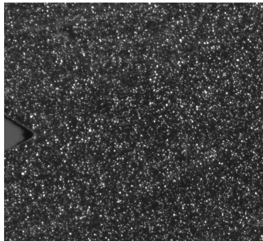
Figure 2. Speckle pattern created on specimen surface
