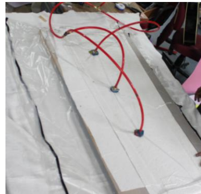
Figure 10. Sealed vacuum layup
