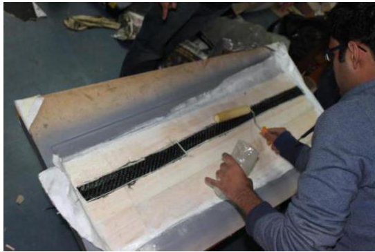
Figure 9. Composite layup using carbon fibre
