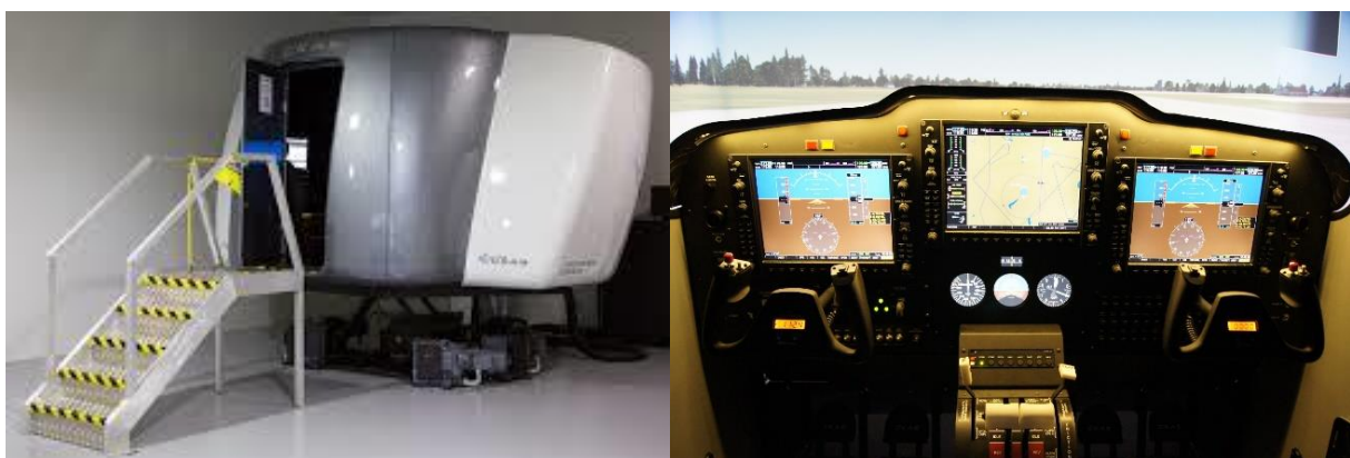
Figure 2. CKAS Motion Sim5 simulator, outer and inner view [14]
