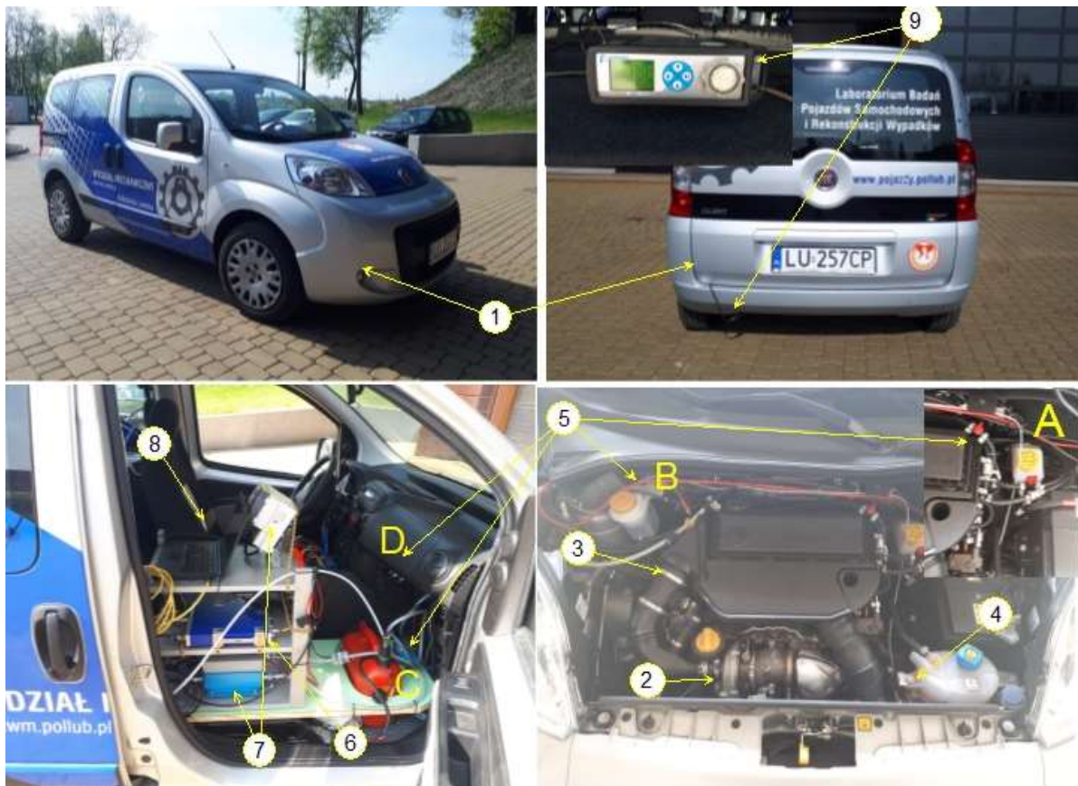
Figure 4. The mobile research stand: 1 Fiat Qubo with a 1.3 Multijet 2 engine. 2. The place of the AVL sensor installing – glow plug socket for the first cylinder. 3. Measurement pincers – obtaining the control signal with the first cylinder injector 4. The spot of receiving the signal of the GMP sensor – inductive sensor. 5. The elements of the additional fuel system – A. Valves, B. The transmitter with the fuse controlling the additional fuel pump. C. Additional exchangeable fuel tank. D. The switch of the additional fuel system. 6. The measuring AVL module and the AVL Universal Pulse Conditioner
