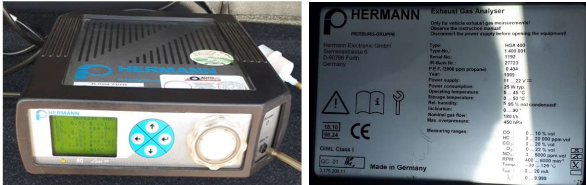
Figure 3. The mobile exhaust gas tester – Herman HGA 400 and its technical specification.
