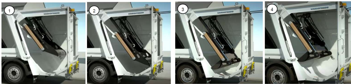
Figure 2. Operation stages of a compaction mechanism
