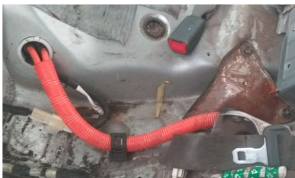
Figure 5. The high voltage cable of the Toyota Prius of the second generation
