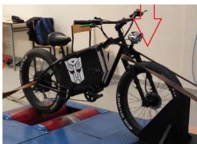
Fig. 1. Two-wheeled electric vehicle during tests on the chassis dynamometer
