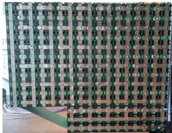
Fig. 2. Connections of cells in the battery pack
