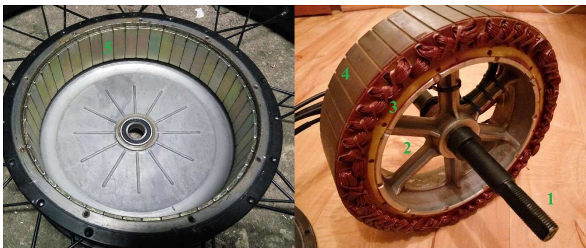
Fig. 3. Photos of the rotor and the stator respectively of the Mxus 3K-Turbo motor.
