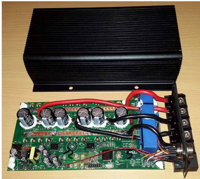
Fig. 5. Photo of the Sabvoton SVMC072080 controller without casing
