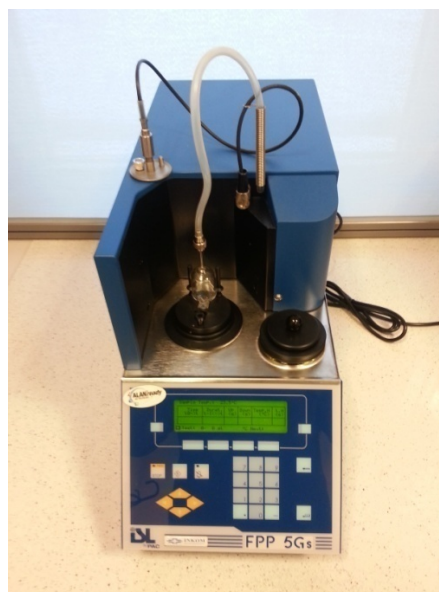
Figure 1. FPP 5Gs automatic device for determination of Cold Filter Plugging Point
