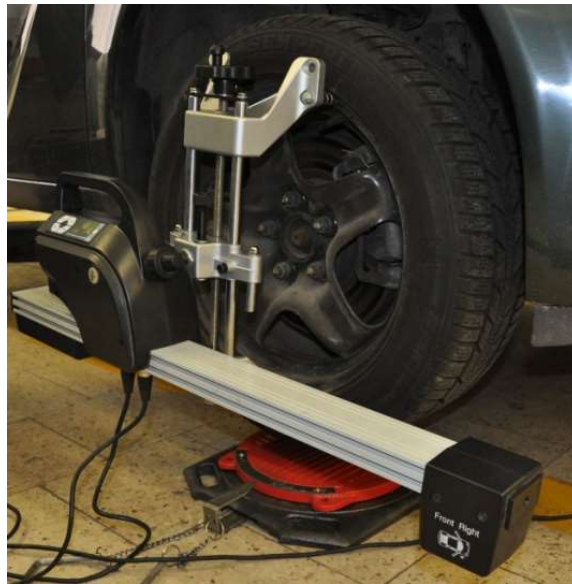
Figure 3. A close-up view of a front right head of the CUSTOR HWA G58 device mounted on a wheel of the tested car
