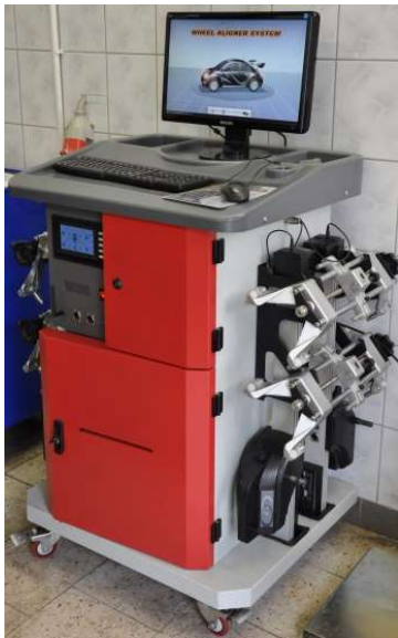
Figure 2. An overview of the main unit of the CUSTOR HWA G58 device. Two of four heads with CCD cameras and the wheel clamps are visible
