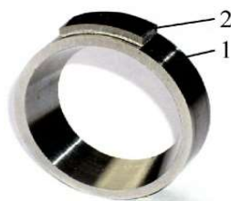
Figure 1. Friction pair; 1-ring sample, 2 counterpart
