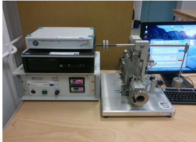
Figure 2. T-20 Abrasive Testing Machine workstation.
