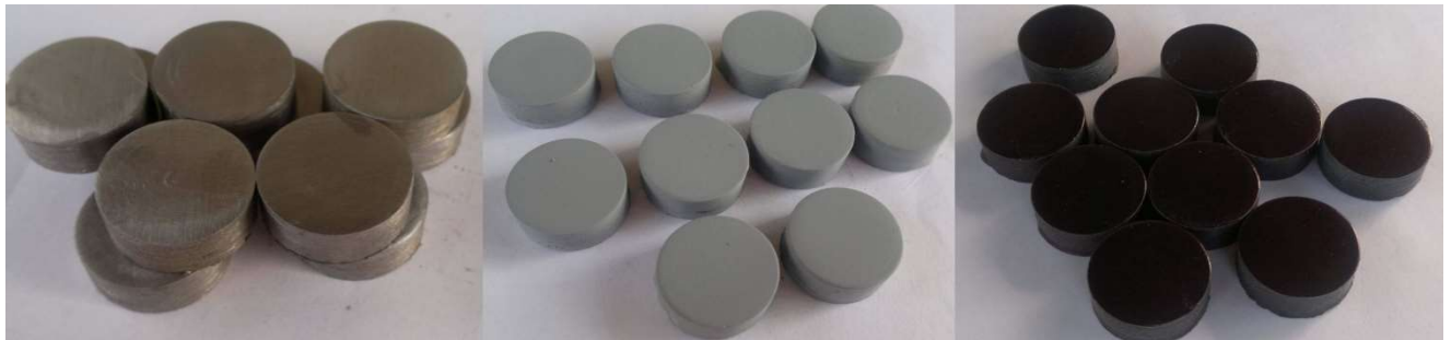
Figure 1. Photograph of samples at each stage of preparation: a) cut and sanded samples b) samples with primer coating, c) samples with basecoat and clearcoat
