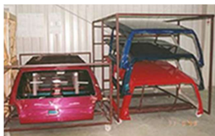
Figure 2. Prefabricated parts of the car body produced in RTM process [16].
