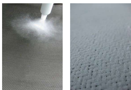
Figure 4. Applying A.S.SET resin powder on reinforcement [20].
