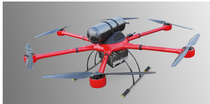
Figure 9. MMC's HyDrone 1550 multicopter equipped with 1800W H1-Fuel Cell [16].
