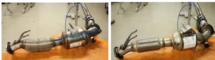
Figure 2. Measurements in a laboratory test facility: original part (left), prototype A (right).
