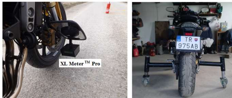
Figure 2. Fixing the console with the XL Meter™ Pro and the auxiliary wheels
