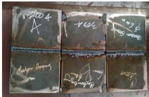
Figure 2. Welding result on A282 Gr C steel
