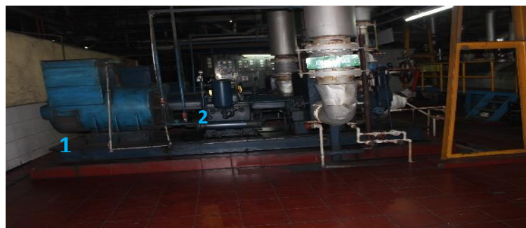
Figure 1. Variation of engine speed is measured at four points of measurement that is at 2 points on the steam turbine generator stand.
