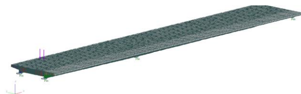
Figure 5. FEM of the bridge
