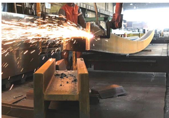
Figure 17. Weld preparation of bended beams at ArcelorMittal Beam Finishing Center.
