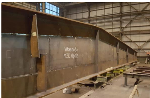
Figure 11. Steel girder using two T-sections and welded-in plate of bridge in Niemodlińska street in Opole.
