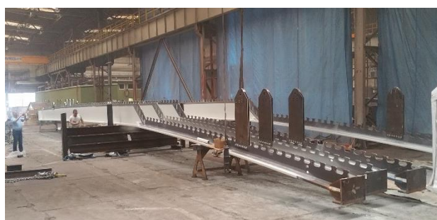
Figure 4. Steel part of PreCoBeam for WA-352, made from rolled sections HL1100.
