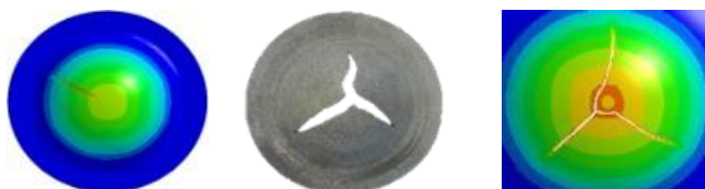
Figure 8. The failure shape of EBE simulation with damage (right) is closer to experimental shape (middle) than without damage (left).
