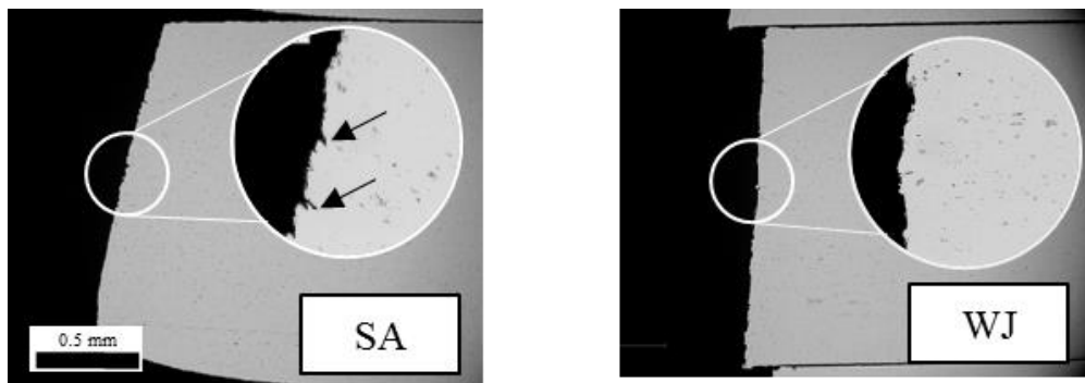
Figure 3. Edge roughness comparison details. 21% shear (SA) to Water-Jetting (WJ) showing acute surface pits on SA sample compared to the smooth undulations of WJ. Insets shown at 1000x original magnification.
