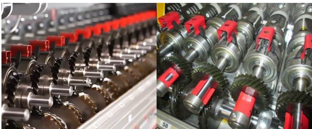
Figure 2. Blank transmission system through roller drivers.
