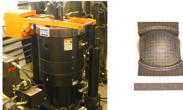
Figure 4. Photograph of the press equipment used for conducting LDH tests and a formed sample.
